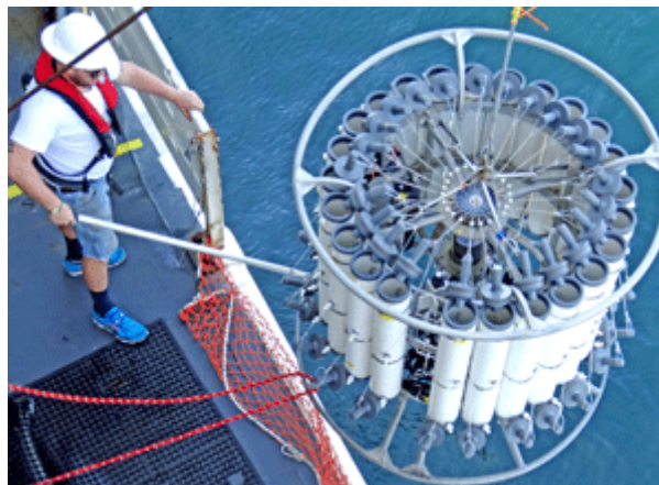
Figure 8 – CTD probe surrounded by a rosette of Niskin water sample bottles
